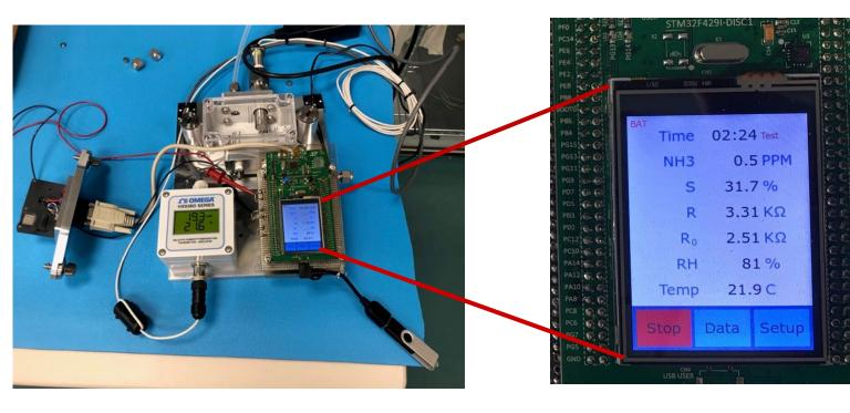
Ammonia and TMA Sensor Setup with **On-Board Temperature and Humidity Sensor**
