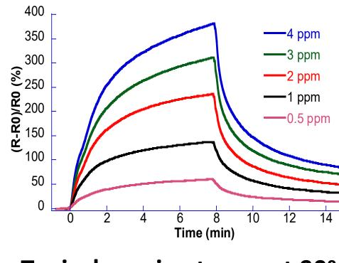
**Typical sensing traces at 90%** humidity: Initial slope is proportional to  $NH_3$  / TMA gas concentration
